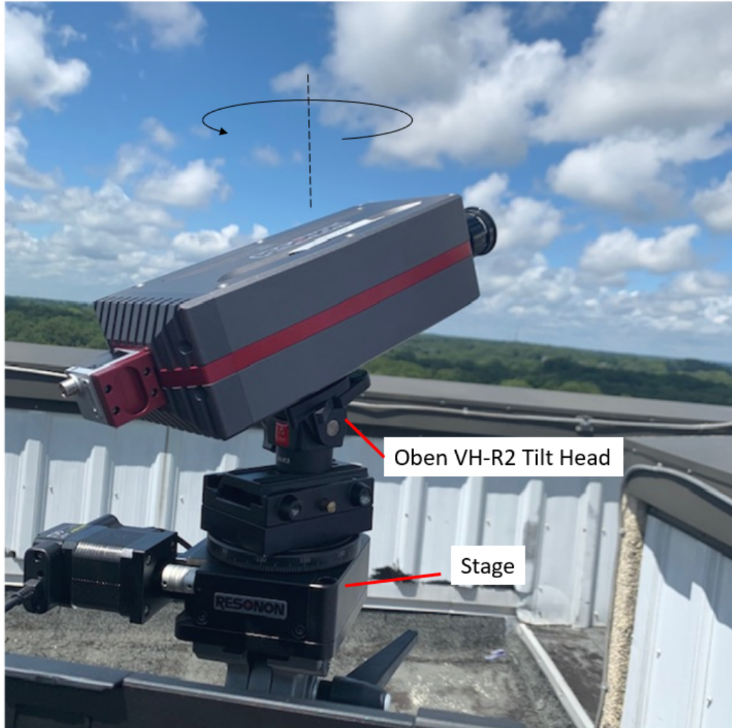
Figure 2.2 Camera stage and tilt head
